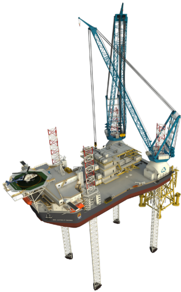
Large deck space with cantilever in parking position
