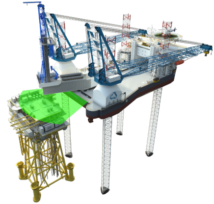
Working envelope rig with patented skidding system
